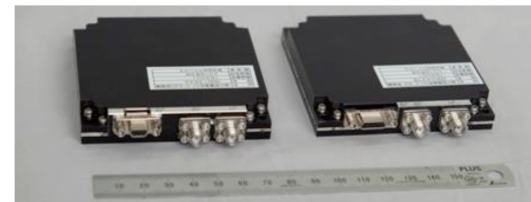
Typical CubeSat RF Transmitter and Receiver © Addnics corp.
